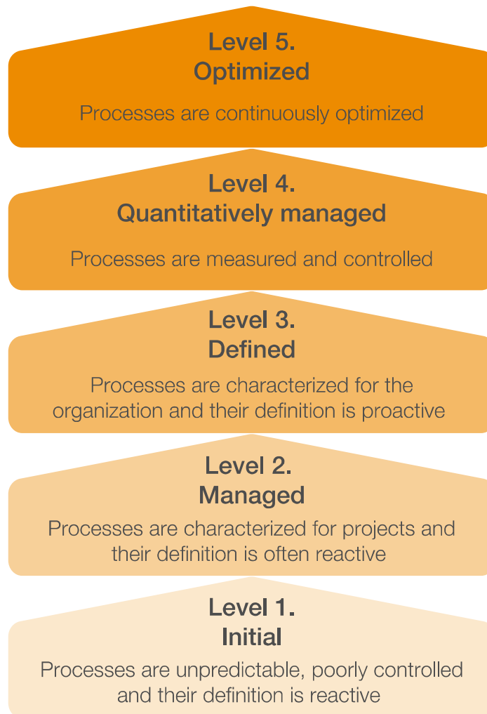
Figure 3. Outline of the capability maturity model. Originally developed at Carnegie Mellon University and now administered by the CMMI Institute
